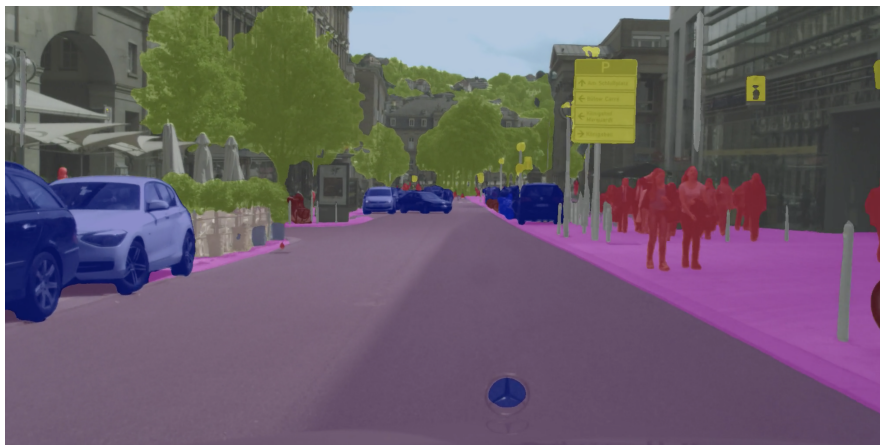
Figure 86: Semantic segmentation of a street scene: a convolutional network predicts the class of each pixel (car, pedestrian, road, sidewalk, vegetation, sign, ...). Result obtained with the GridNet architecture (Fourure et al., 2017).
